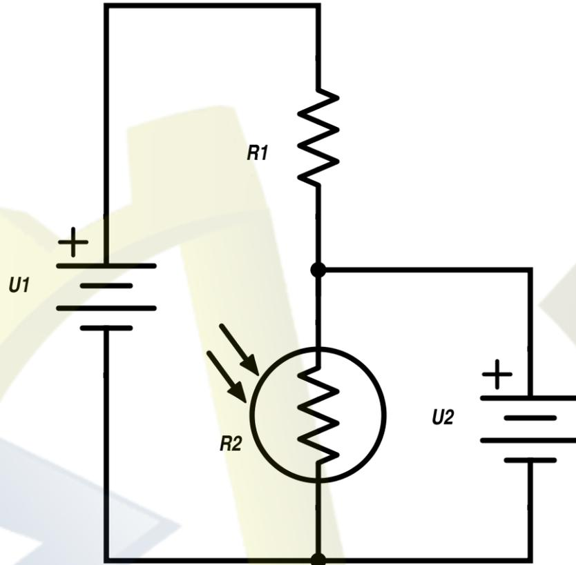
Fig. 3 Voltage Divider Application
