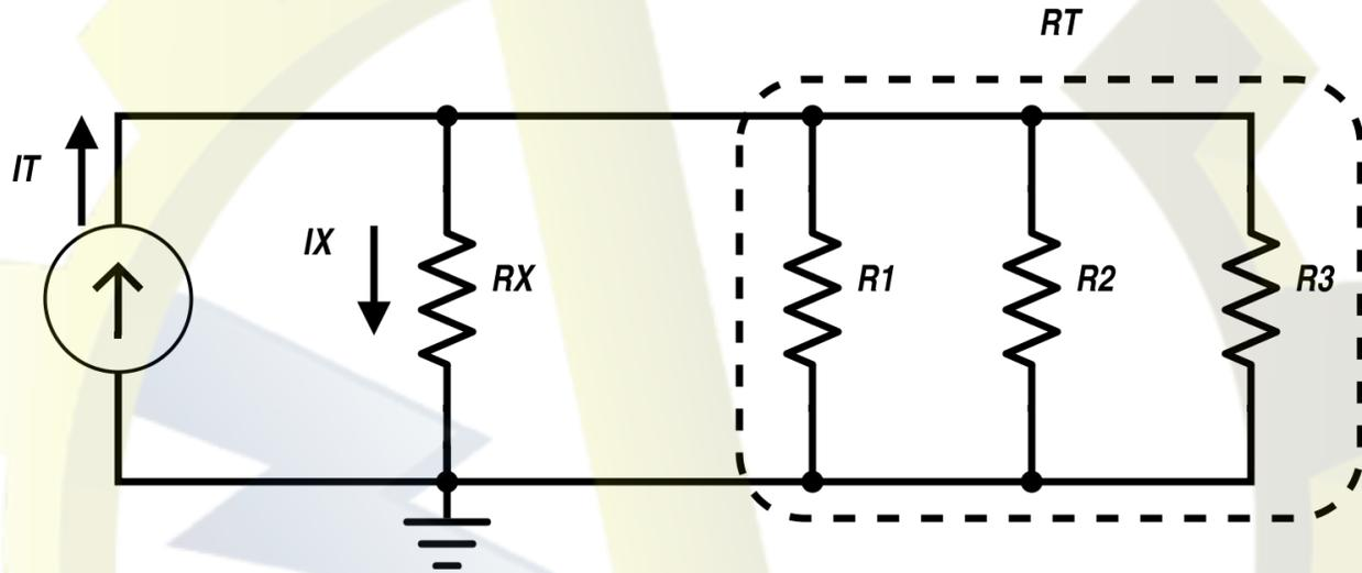
Fig. 2 Current Divider Circuit
