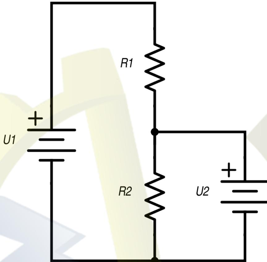
Fig. 1 Voltage Divider Circuit
